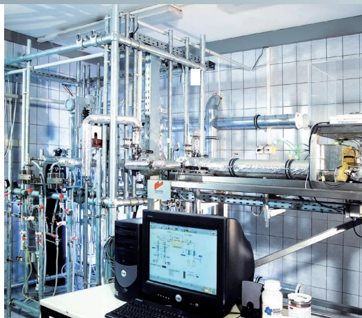
Vogelbusch test equipment for adsorption process research
